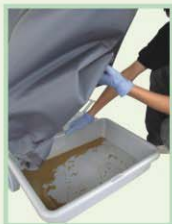
Support tray prevent liquid spilling on floor 托盤可避免廢水滴落地面
